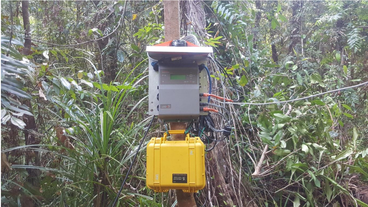
Figure 14: A recording unit of the ALS set up in Suaq Balimbing. On top (black) is the GPS device for time-synchronization, a metal cover shields the recorder from rain and falling debris. The recorder (Song Meter SM3, Wildlife Acoustics Inc.) is connected via cable to a SMX-II microphone deployed in 10 m height in the canopy and is powered by a 12 V, 18 Ah dry gel battery (inside yellow case). The battery was charged by a 50 W solar panel. (Photo credit: Urs Wipfli, 2017)
